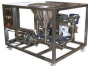
Blender is compact, it consists of a centrifugal puma with a ventury system at the suction side and a hopper with a butterfly valve at the upper part to add solid media to the pumped liquid. Depression is created at the base of the hopper due to the ventury and suction systems of the pump.
