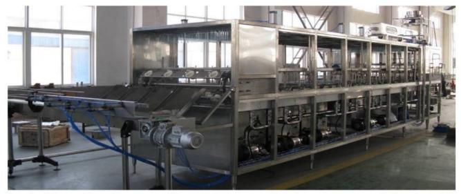
Linear jar filling machine adopts pressure filling way. Product water flows into water storage tank through regulating valve. The pipes of long diameter and
