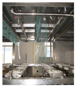
Automatic Jar inside washing machine is exclusively used in washing 20 liter on inside of Jar. The production line can do automatically washing, sterilizing, with a good appearance, easy operate, low-loss energy & save water, high working efficiency. The frame of the machine is welded by 38 x 38 stainless steel square tube, with the characteristic of high intensity, good rigidity, light weight, aesthetic appearance, easy washing etc.
